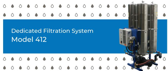
The Model 412 fits eight COMO Filters, giving it the filtration capacity needed for large reservoirs while maintaining 1  $\mu$ m particle and 20 ppm water performance. Each filter holds up to 20 pounds of dirt and 1 gallon of water, so COMO can help you extend fluid life and reduce downtime with fewer filter changes than the competition.
