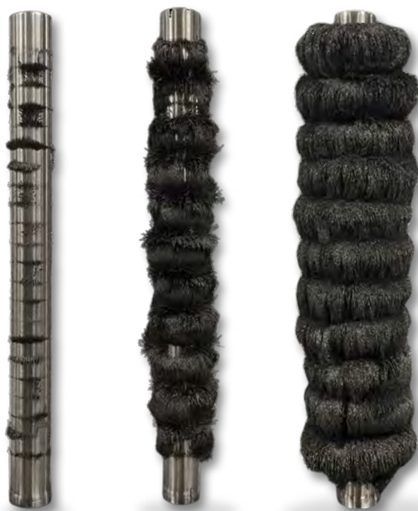
1" magnetic filter elements with varying loads of contamination. Dirt holding capacity*: 3.97 lb-ft.
